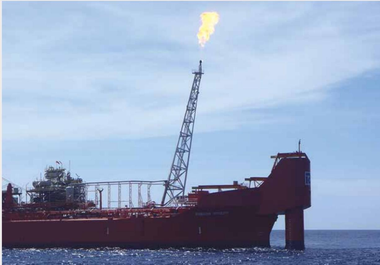
**Orwell Offshore's standard packages include a harsh weather external column turret suitable for integration with a converted or new build FSO/FPSO.**
